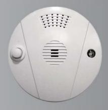
HD-9ZW is Z-Wave enabled heat detector with both rate-of-rise and fixed temperature sensors. Adopting Z-Wave as its communication protocol, the detector is compatible with any Z-Wave devices and Z-Wave mesh networks.
